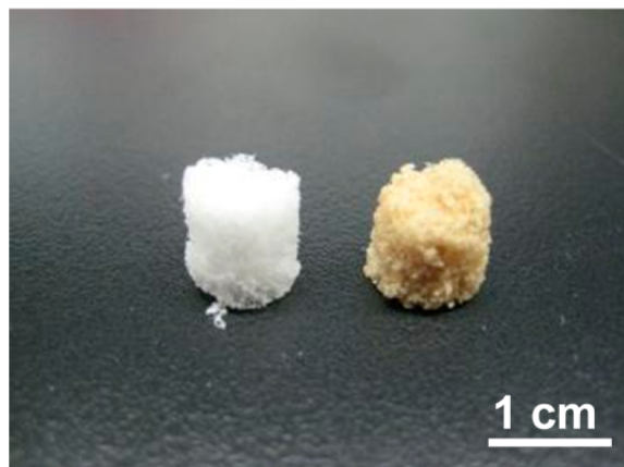
Figure 1. (Left) photograph of an untreated PDLLA scaffold. (Right) photograph of a P-PDLLA-2h scaffold. The color change is due to presence of azo bridges ( -\text{N}=\text{N}- ) on the scaffold.
